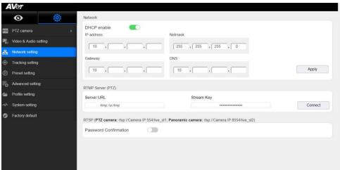
\*Note: It is a good idea to verify the Gateway/DNS of your network; this is how the camera stream will access the WWW.
