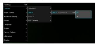
After turning DHCP on, go to **Information** to view the IP address.
