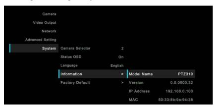
2. Once you have the IP address setup, type the IP address in your Chrome browser (Setup on same subnet) and you should now see the login to the PTZ330 camera shown below.
