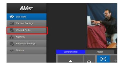
5. Next, after selecting the *Video & Audio* setting, verify that you have either "Stream Only" selected or "USB + Streaming" selected, depending on your setup. Select your Stream Video Output standard, Bitrate, Framerate, Encoding, etc.
