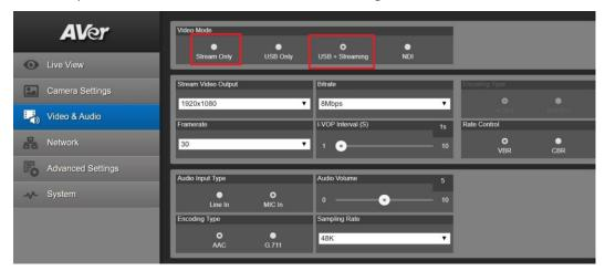
\*Note: Once streaming has started do not change the Stream Video Output on the fly, you will need to "STOP" streaming, change the Stream Video Output, then "Start" the stream again.
